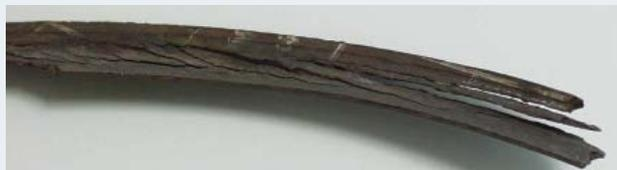
◀ Over-compression created concentric splitting throughout the compressed portion of this gasket, crushing it.
