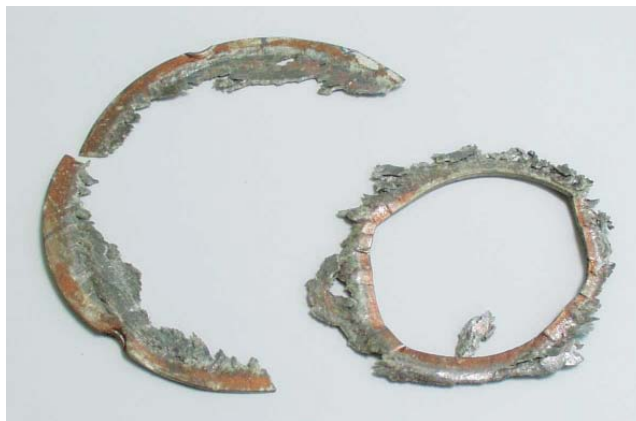
▲ Figure 3. The wrong lubricant reduced this gasket’s retentive friction on the flange, allowing it to extrude, softening the EPDM binder, and reducing the gasket’s crush strength.
