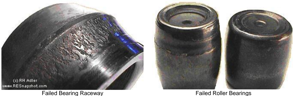
Figure 1 – Failed Roller Bearing Elements
