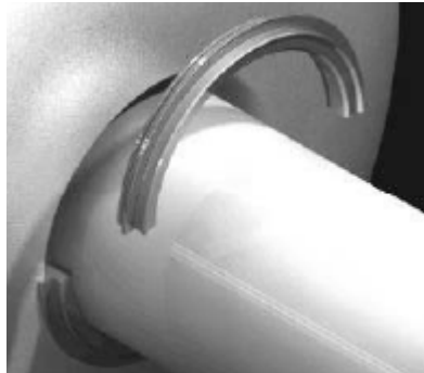
PLACE SPLIT HALVES OF STATOR AROUND SHAFT
