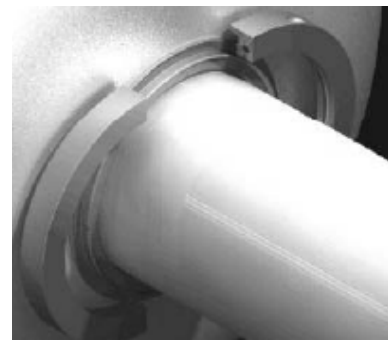
SLIDE ROTOR HALVES AROUND SHAFT
