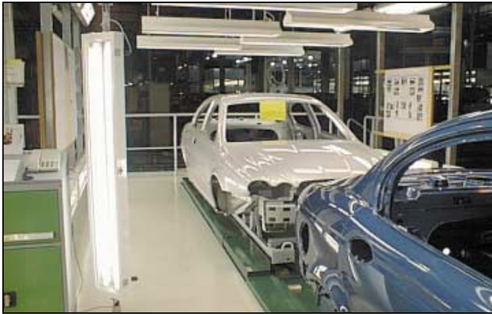
Finished body shells ready for assembly at the Halewood Jaguar plant.
