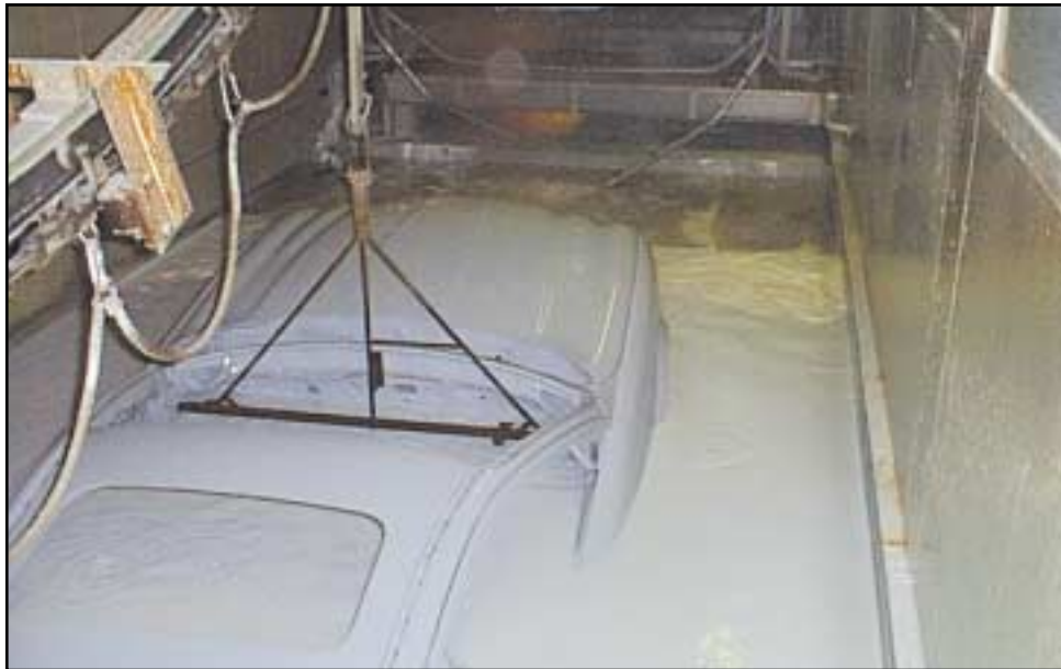
Sealing "E Coat" at the Halewood jaguar plant.
