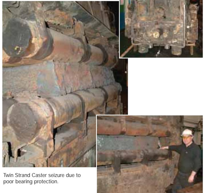
Twin Strand Caster seizure due to poor bearing protection.
