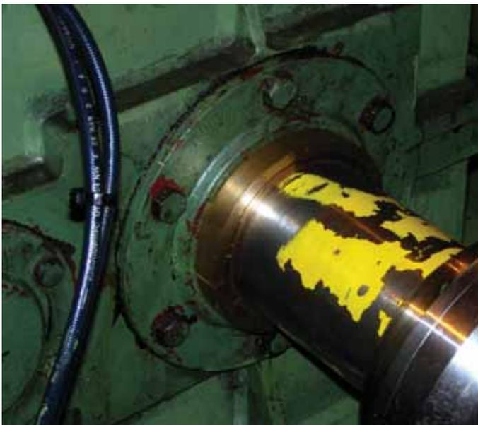
Case Ref: 3370 - 100mm LabTecta-RDS™ (Split seal) working on gearbox at 1,500rpm
