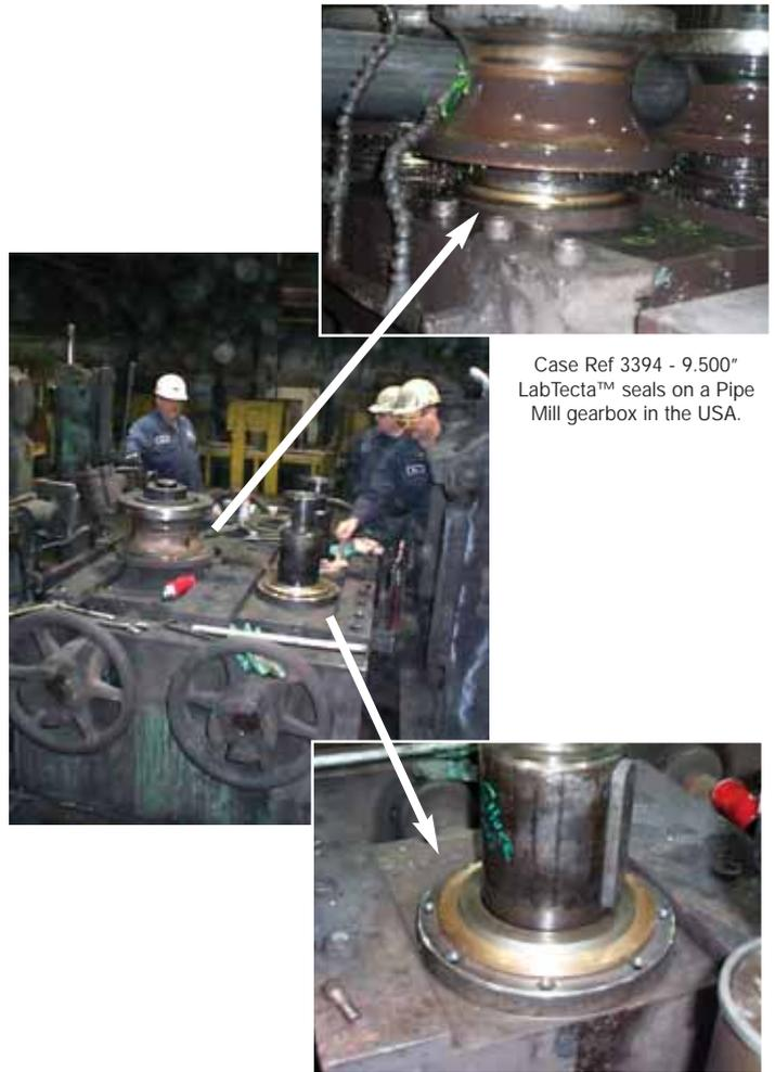
Case Ref 3394 - 9.500" LabTecta™ seals on a Pipe Mill gearbox in the USA.
