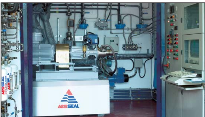
API 682 Hot oil cell (240°C/464°F). - One of FIVE state of the art test bays at AESSEAL® headquarters.
