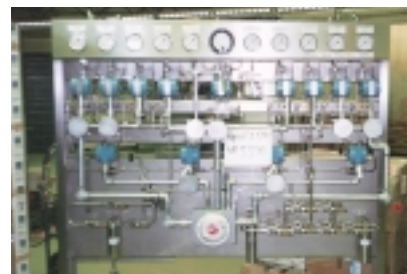
Tubed Panel – 316 ss Tubing
