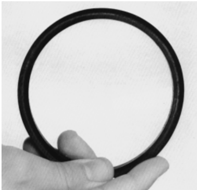
Figure 1. This Kalrez V-ring was essentially unaffected by six years downhole.
