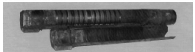
Figure 2. Tubing-to-packer seal after six years downhole
