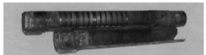
Figure 2. Tubing-to-packer seal after six years downhole
