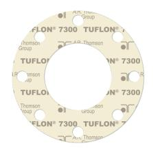
TUFLON® 7300 is a barium sulfate filled PTFE gasket material, specifically formulated for service in strong caustics, moderate acids, chlorine, hydrocarbons and cryogenics. TUFLON® 7300 is highly resistant to creep relaxation and has outstanding sealability characteristics. The product can be supplied with FDA compliance.
