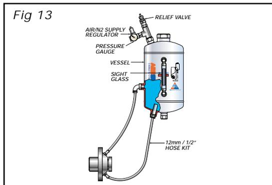
Air/Nitrogen Pressurized Barrier System SSE10™ P2
