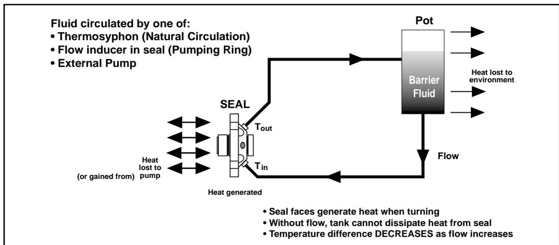
Fluid flow in Double Seal Barrier System
