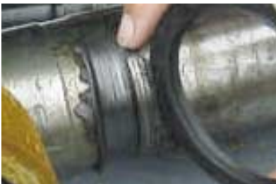
Shaft Damage from a Lip Seal
