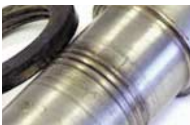
Shaft Damage from a Labyrinth Seal
